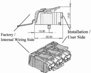
Installation / User Side Factory / Internal Wiring Side Wiring Holes (a)+(b) Wiring Holes (a)+(b)
